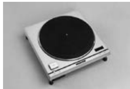
Fig. 12.10. Matsushita direct drive turntable SP-10 (1970) (10)
