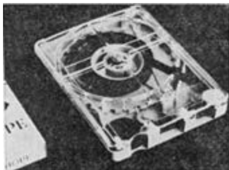
Fig. 6.3. Fidelipac cartridge (1962) (3) 102 x 133 x 24 mm four-track/two channel
