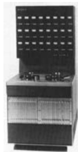
Fig. 14.5. Sony 24-channel stationary-head DAT prototype (c. 1977) (4)
