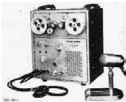
Fig. 4.9. NEC MR-1 steel wire recorder (1948) (9)
