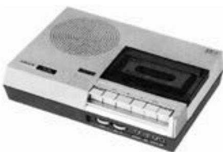
Fig. 6.11. Sony TC-1160 (1968) (11) The first machine with an inbuilt electret condenser microphone
