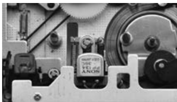
Fig. 6.17. TCM-280 erase head, recording/playback head
