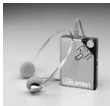
Fig. 13.3. Sony WM-2 (1981) (3) The first Walkman specifically designed as a “headphone stereo”
