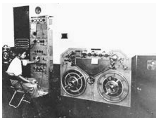
Fig. 3.10. Marconi-Stille steel ribbon recorder (1937) (9)
