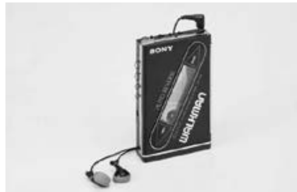
Fig. 13.6. Sony WM-101 (1985) (6) The first machine to have a gumstick battery
