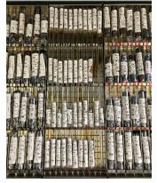
Creep ruptured specimens
