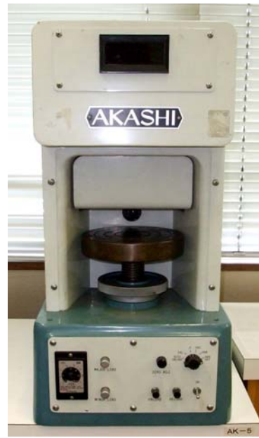
(3) Standard Rockwell Hardness Tester (NRLM-Akashi Type)
