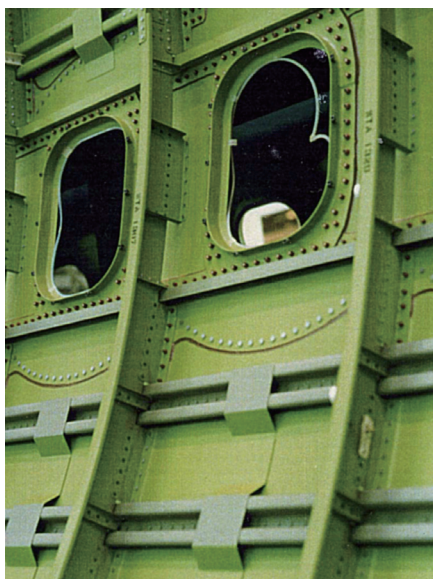
Figure 10.15 Boeing 767 Fuselage with Tapered Rolled Stringers 31, 32
