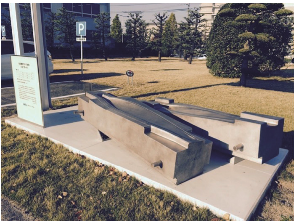
Figure 5.16 Forging Die for Aircraft Propeller Stored at UACJ
