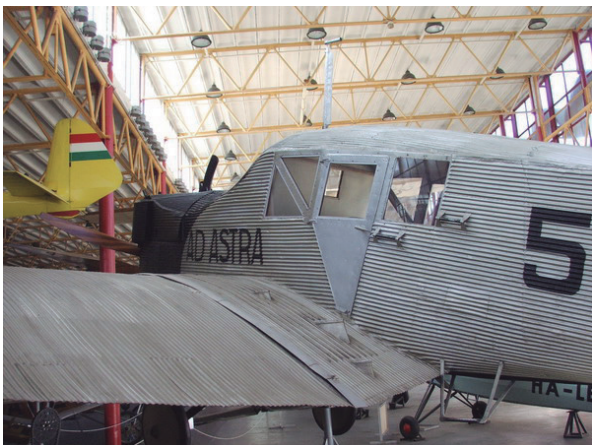
Figure 4.9 Junkers F.13, All-Metal Passenger Plane Using Corrugated Duralumin (©2006 Andi Szekeres) 16
