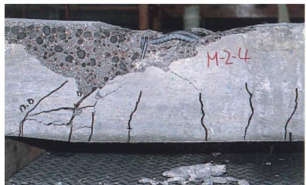
Fig. 6.10 Concrete strength test under low temperatures, photograph.<sup>6-7)</sup>
