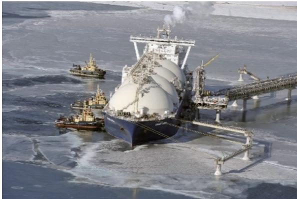
Fig. 3.9 Icebreaking LNG carrier and ice-resistant port facilities (Port of Prigorodnoye, Sakhalin), photograph.<sup>3-12)</sup>
