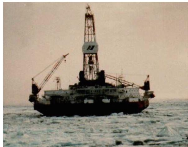
Fig. 8.6 *Kulluk* (drill barge), reverse conical floating structure, photograph: Built by Mitsui Engineering & Shipbuilding Co., Ltd., 1983.<sup>8-1)</sup>
