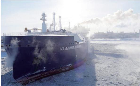
Fig. 9.8 World's first icebreaking LNG carrier, *Vladimir Rusanov*, photograph: Daewoo Shipbuilding, South Korea, Dec. 2017; maximum icebreaking capability, 2.1 m (in reverse).<sup>9-8)</sup>
