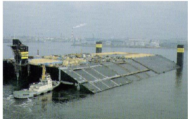
Fig. 8.9 Submersible barge MAT, constructed for SSDC, photograph: Innovative structure—steel layers bonded using high-density urethane.<sup>8-1)</sup>
