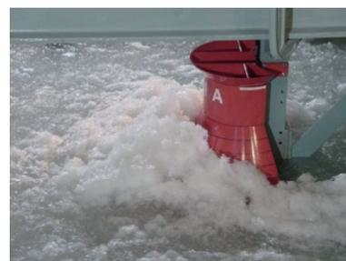
Fig. 1.2 Experiment to measure ice force against a structure, photograph.<sup>1-1)</sup>
