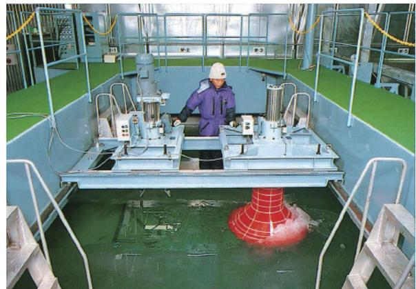
Fig. 6.9 Ice load test on a conical wall structure, photograph.<sup>6-7)</sup>
