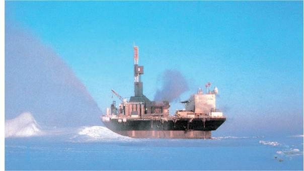
Fig. 8.17 Super CIDS mobile artificial island in operation, Beaufort Sea, Alaska, photograph.<sup>8-8)</sup>
