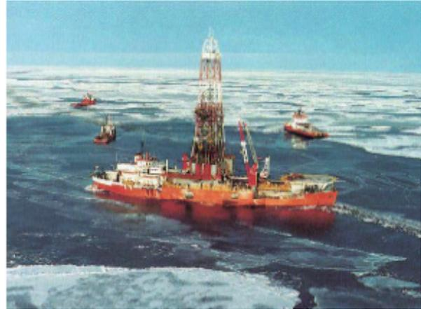
Fig. 8.5 Floating drillship, photograph: Support vessels needed to remove sea ice to lessen impact on the drillship.<sup>8-1)</sup>
