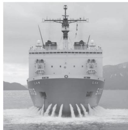
Fig. 9.5 Second *Shirase* icebreaking enhancement—Sprinkler system, photograph: System sprays water from bow nozzles to reduce friction between snow/sea ice and the ship.<sup>9-2)</sup>
