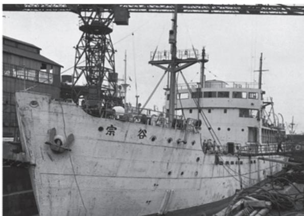
Fig. 9.2 Lighthouse supply ship *Soya* at start of conversion into an Antarctic research vessel, photograph.<sup>9-4)</sup>
