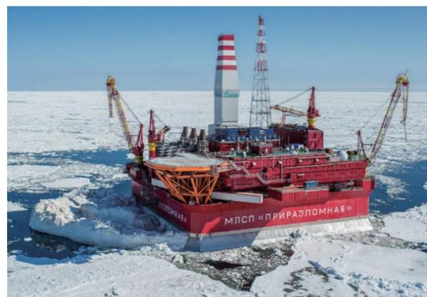
Fig. 3.8 Ice-resistant oil production platform operating on the Russian arctic continental shelf, photograph.<sup>3-11)</sup>
