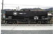
(4)JAPAN FREIGHT RAILWAY "HOKI-5700"TYPE(No.25767) 40TON CEMENT HOPPER CAR
