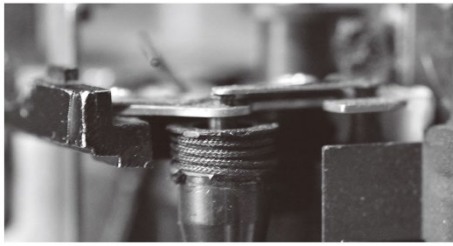
Photograph 6-43 Olympus Shutter Structure
