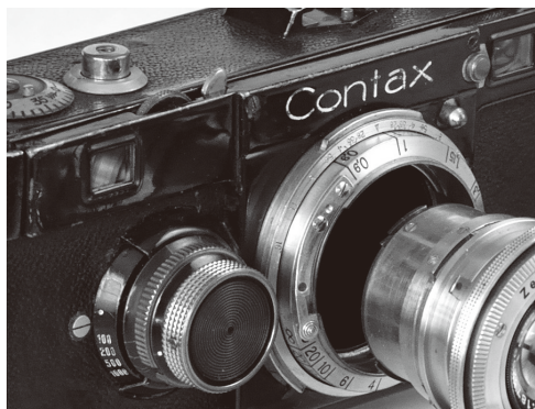
Photograph 4-7 Lens Mount of the Contax
