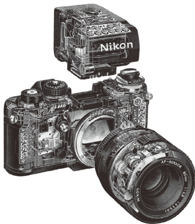
Figure 6-21 Perspective View of the Nikon F3AF 22)
