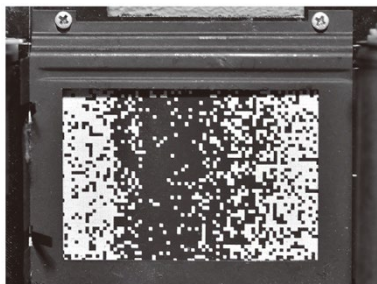
Photograph 6-11 Printing Pattern for Curtain Surface Metering of Olympus
