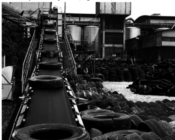
Fig. 9.3 Cement Kiln Whole Tire Conveying Device 3)
