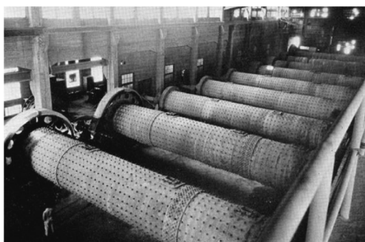
(1) Finishing Mills Installed in 1932 (637kW)
