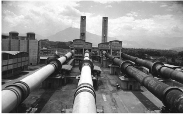
Fig. 4.5 Photograph of a Wet Process Long Kiln (Kiln Length 170m) 7)
