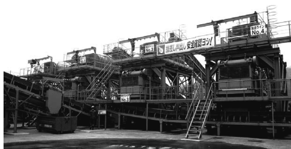
Fig. 9.10 Disaster Waste Desalination System at Taiheiyo Cement’s Ōfunato Plant (photographed by the author)
