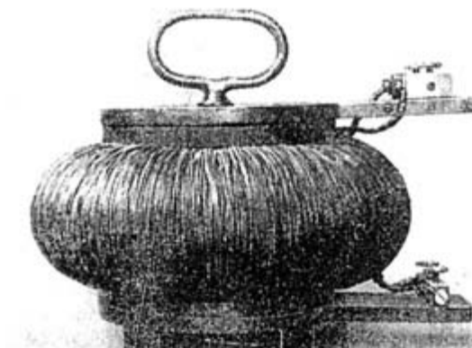
Photo 3.2. The Shell-Type Transformer Displayed at an Exhibition in Budapest by Ganz (1885)
