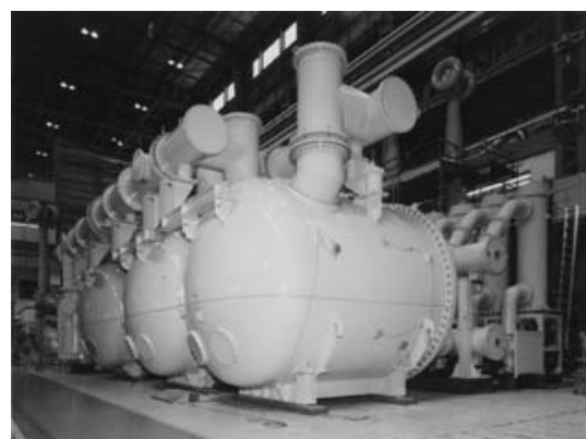
Photo 5.13. A Gas-Cooled, 275kV, 300MVA Transformer for the Tokyo Electric Power Company Higashi-Shinjuku Substation (1994, made by Toshiba)
