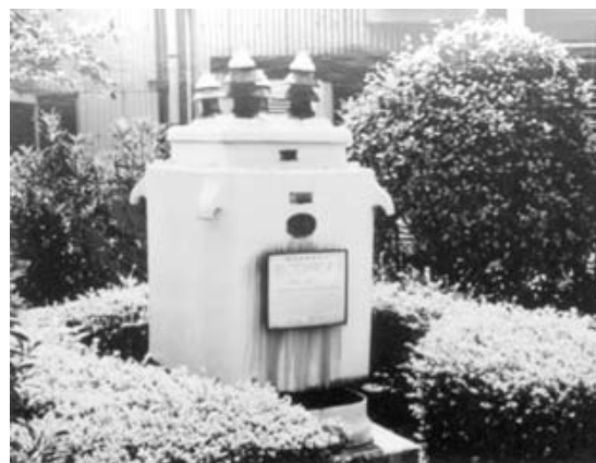
Photo 3.5. The Oldest Extra-High-Voltage Transformer in Existence (13.2kV, 100kVA; made in 1910 by Shibaura for Shinano Electric)
