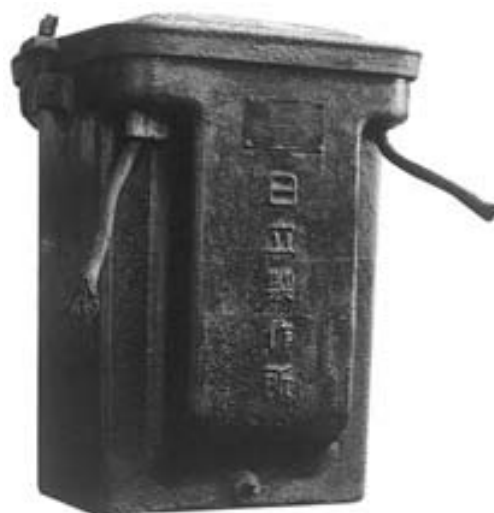
Photo 3.6. 5kVA Transformer for Hitachi Mine (made in 1910 by Hitachi)
