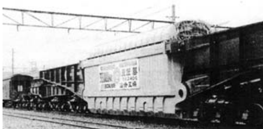
Photo 4.6. A 300MVA Transformer for the Chubu Electric Power Company Nishi-Nagoya Substation, the Highest Capacity Transformer to be Transported (1963, made by Hitachi)
