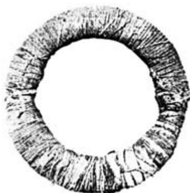
Photo 3.1. A Model of Faraday's Electromagnetic Induction Coil (1831)
